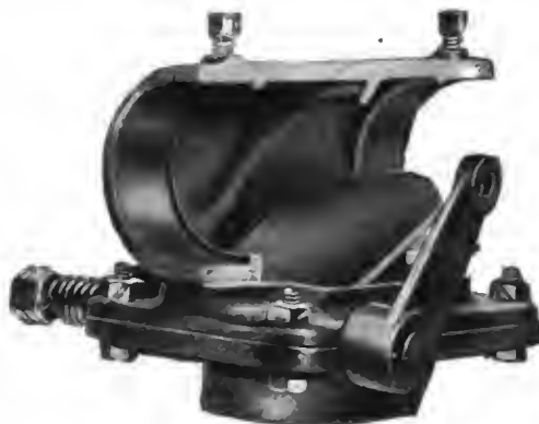
G. P. muffler cut-out in section
